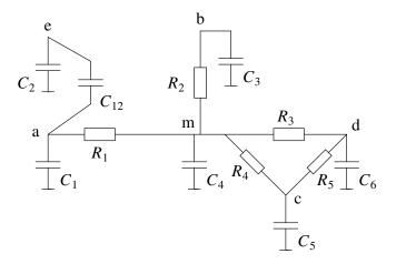
In the above figure, node m corresponds to the piece of metal that connects the three different poly branches. If also metal resistances are extracted, or if no network reduction heuristics are applied, this node will not be present.
