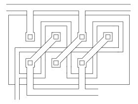
If a field-effect transistor is used as a capacitor and has only one connected set of drain/source areas, two connections will be generated that are however attached to the same net. If a field-effect transistor has more than two drain/source connections, only two of these connections appear in the extracted circuit. (These will in general be the connections that are connected to other parts of the circuit; dangling connections are not used in this case.)
