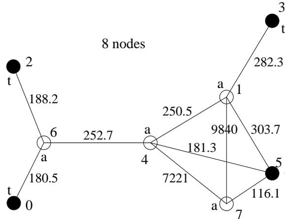
Function *reducMaxParRes* can now try to remove too high-ohmic shunt resistors. It starts in Evaluation loop(1) with the non area nodes. It starts with node 0, this node has only one resistor and does not really to be done. Nodes 2 and 3 have also only one resistor. Node 5 is the last candidate to be node 'n' and to make a clique. Nodes 1, 4 and 7 are placed with node 'n' in the clique (in random order).
