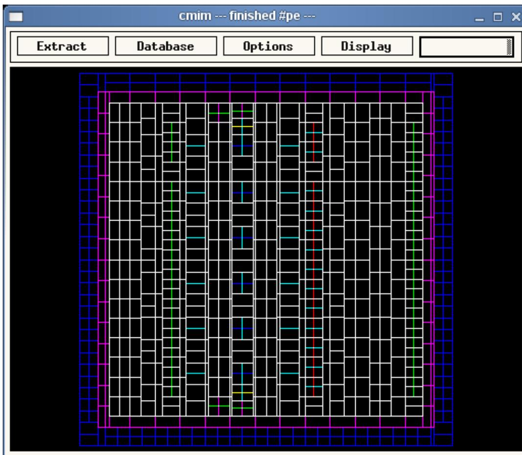
The above picture shows the modified mesh, which gives no problems for "space3d". You see that it is more orthogonal than the mesh of the following picture.
