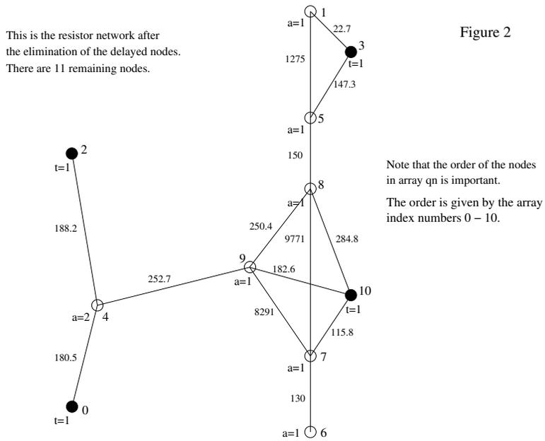
In function `reducGroupI`, we start with the remaining nodes of the resistor network (see figure 2 above). Some special nodes can not be eliminated because they are terminal nodes. The 4 terminal nodes (with `t=1` flag), which are also a pin of a transistor. Note that for the 2 d/s-area nodes (on the left) the nodes touching the gate edge are joined together. And note, that the 2 gate terminal nodes (on the right) are in the top-right position of the gate area (see figure 1 above).
