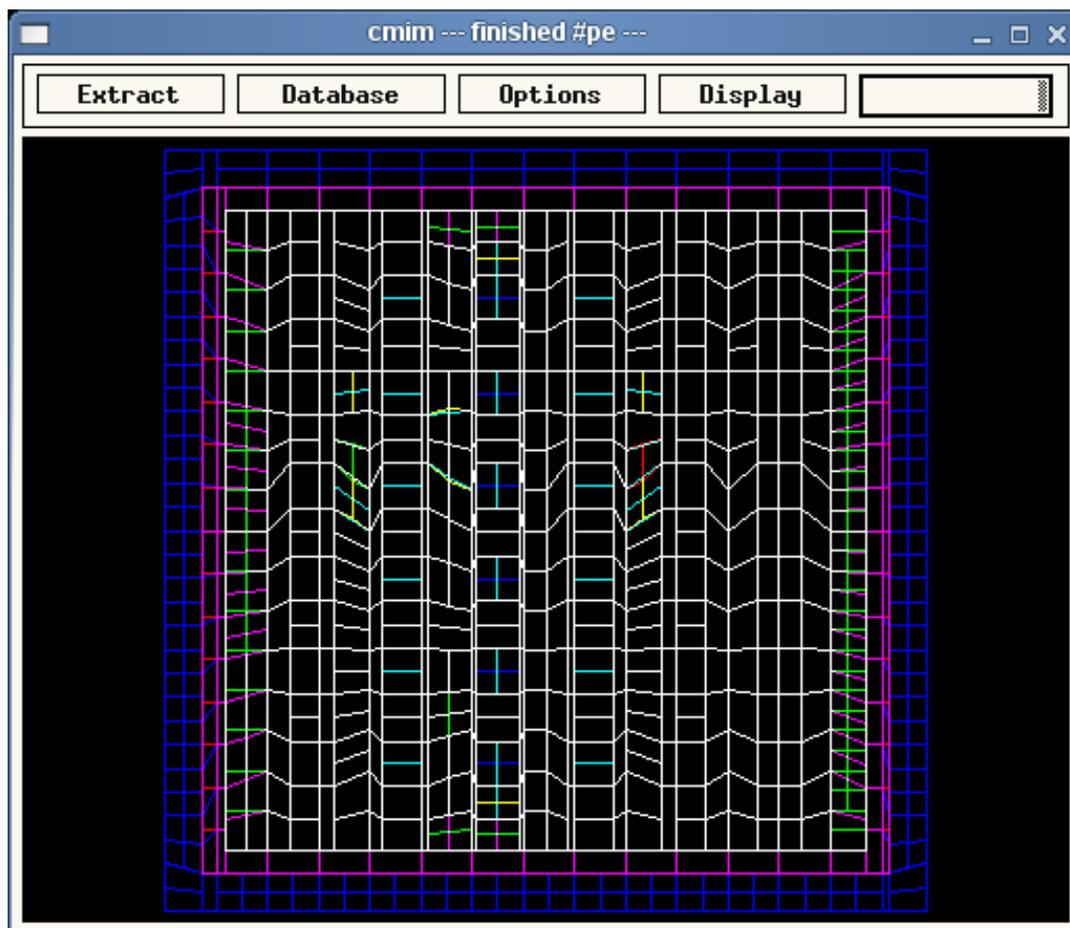
The above picture shows the unmodified mesh, which results in "space3d: Encountered NAN in schur module". This happens when edges are split too far from their original x or y point, because there is already a spider found.
