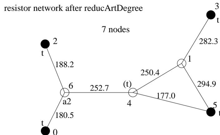
Now, we can again use `reducArtDegree` to eliminate node 1. We get the following resistors: 772.4 (3 - 4), 909.7 (3 - 5) and 145.2 (4 - 5). Note that we can not eliminate node 4, because it has node "names". Note that when `reducMinRes` removes the 42.4 ohm resistor, then also node 4 can be eliminated.
