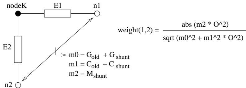
The shunt values between n1 and n2, are the added values when nodeK is eliminated. The branch weight(1,2) is the added moment (m2) divided by cap and res parts. The old values are the existing admittance values between n1 and n2. The old moment is default (sne.errorfunc=0) not used.
