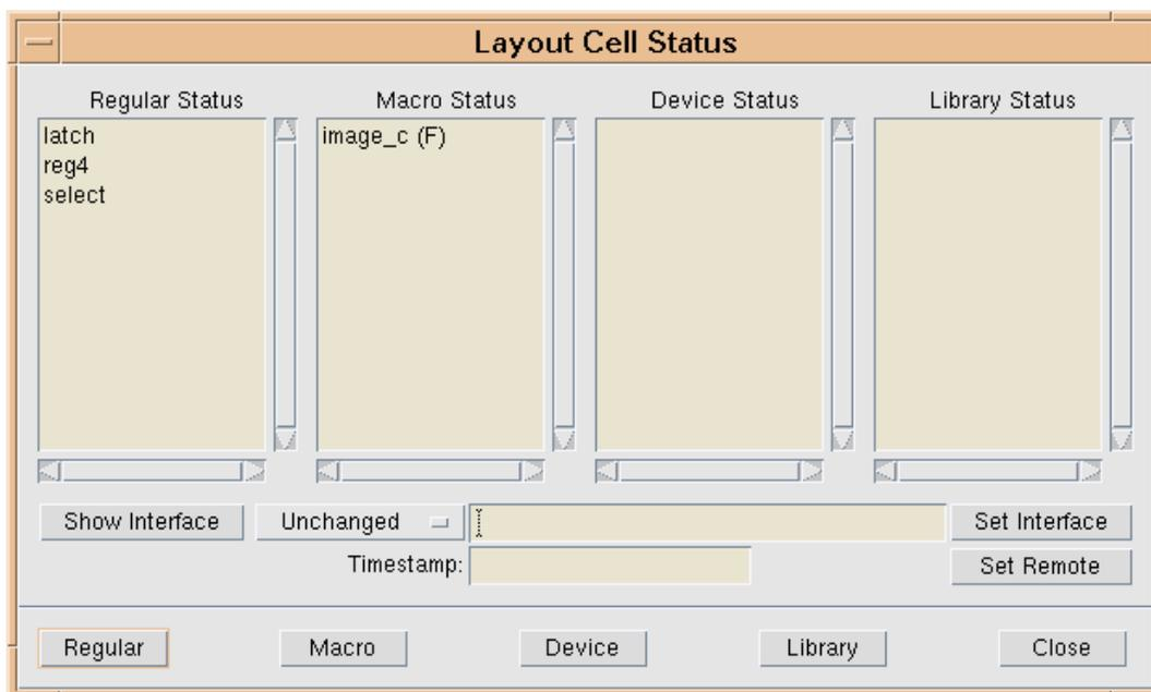
Then, when the circuit is extracted in hierarchical mode, a circuit is produced in which "image\_c" has been flattened but in which the rest of the hierarchy has been preserved.
