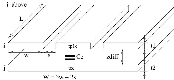
To compute 'Ce', we must do two cap3D extractions of the used layout model. We use two different widths 'w' and 'w2' for the mask 'i' lanes. The length 'L' of the lanes is not changed. For the surface mask 'j' plane, we use a width 'W', which is 3 times the width of the 'i' lanes plus 2 times the used spacing 's'. The formula to compute 'Ce' is:
