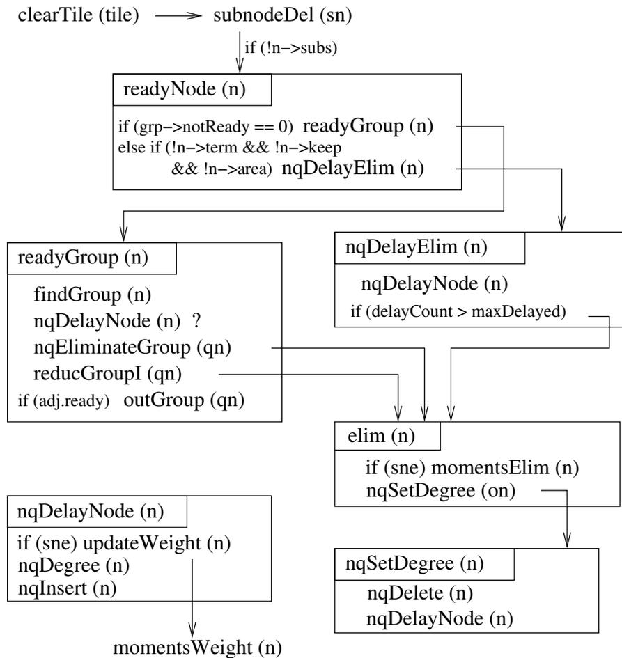
Function `findGroup` places the nodes of the group in array `qn`. After function `nqEliminateGroup` there are not more delayed nodes in array `qn`. Thus, all delayed nodes are removed from the priority queue and possibly eliminated. Note that the eliminated node is not more in the priority queue.
