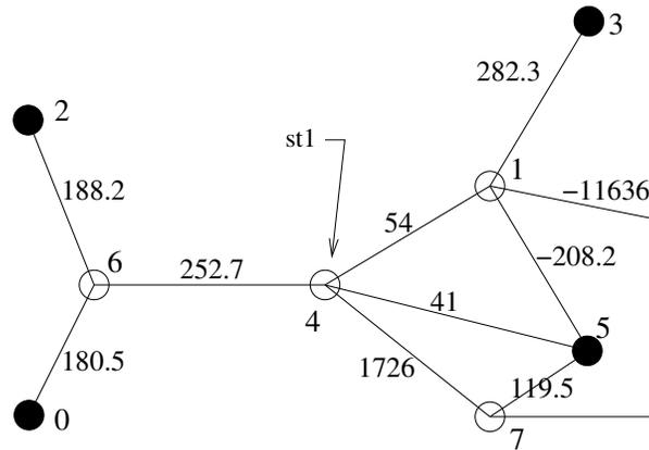
Because of the `nodeJoin` reduction, the other 2 low resistors are still in the network. Thus next `nodeJoin` shall join nodes 1 and 4 and following `nodeJoin` shall join nodes 4 and 5. This gives a dangling node 1 as result:
