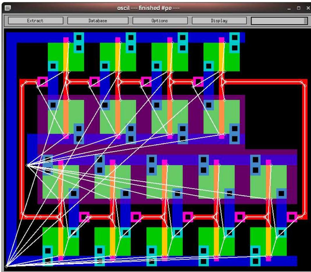
This picture of the demo/suboscil project shows the outputted resistor network.
