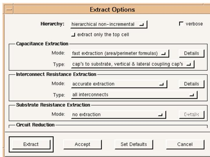
and set extraction mode "Hierarchy:" to "hierarchical incremental", and the "Capacitance Extraction" and "Resistance Extraction" "Mode" fields to "no extraction".
