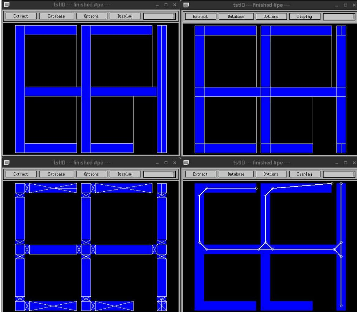
The above pictures demonstrate path preserving. The first picture gives the normally used tiles and boundaries. The first tile on the left side can not have line nodes because it has extra points on its right side. On the right side of the layout you see a tile which is split, because there are terminals defined. The second picture demonstrates what the preprocesses have done. The tiles have get extra splits and two stopping boundaries are layed done to stop the terminal splits.
