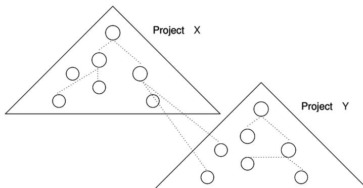
As one can see, some of the cells in projects X and Y are defined hierarchically, instantiating local cells. Project X however also contains cells which instantiate cells from project Y. These remote cells have been imported previously into project X, before instantiating (= referring) them within this project.
