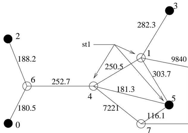
When we want, that st1 is joined with node 5, then we must change the code of function `reducMinRes`. Because the node with lowest resistor value is the best candidate.
