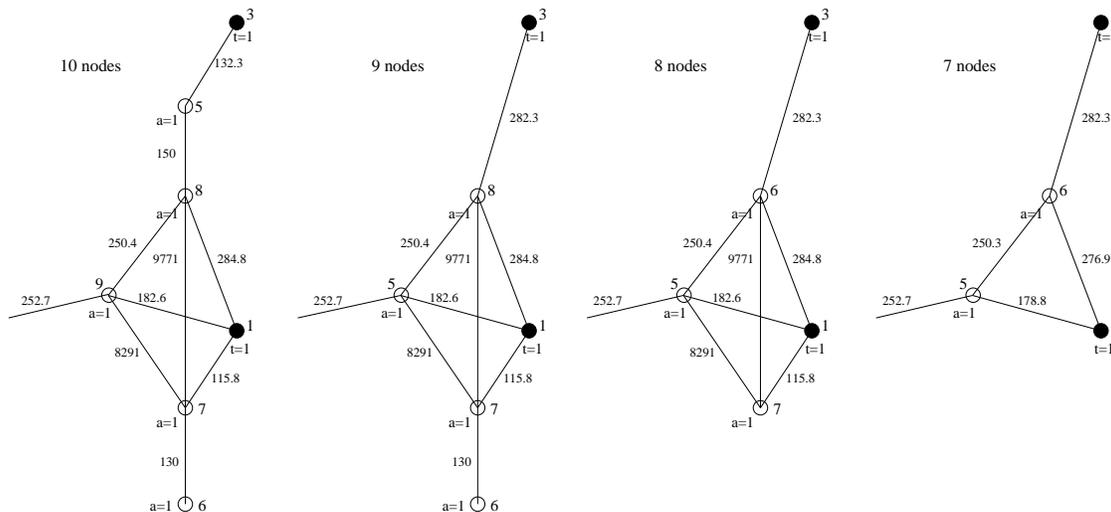
Finally, node 7 can be eliminated, because its `degree=3` < `min_degree`. This results in 7 nodes. Because nodes 5 and 6 are not more evaluated, they are not eliminated. But when another initial node order in qn was used, at least 1 more node could be eliminated.
