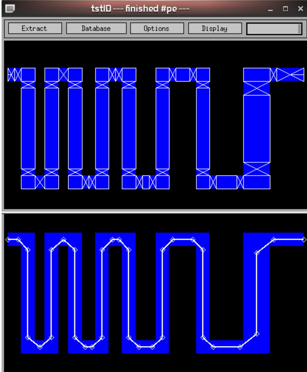
Another example of path preserving. Depending on the distance not always two special nodes can be used. By the terminal node on left top a node is preserved very close to it. On the right side you see that a different path delta-x gives also a different height of the special equi-line rectangle.
