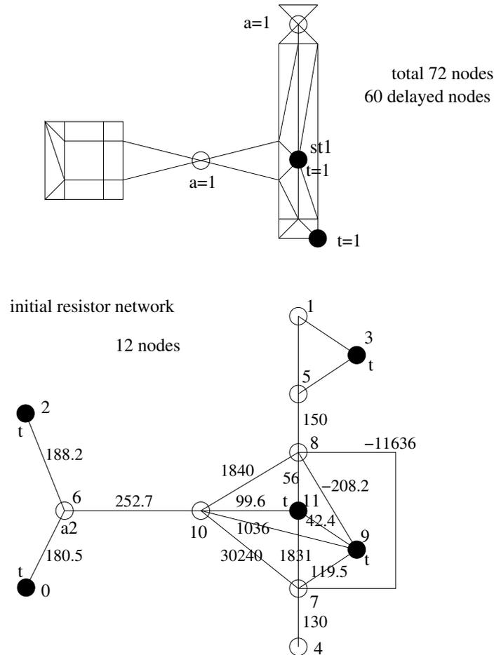
Function `reducArtDegree` can eliminate 3 nodes from the above initial resistor network. The following nodes: node 1 (node 11  $\rightarrow$  1), node 4 (node 10  $\rightarrow$  4) and node 5 (node 9  $\rightarrow$  5). This results in a 282.3 ohm resistor between node 3 and 8 and nine remaining nodes.
