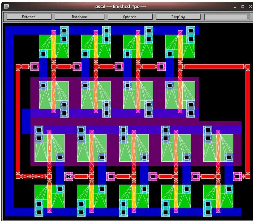
This picture is made of the demo/suboscil project and shows the resistivity mesh. You see that only the poly interconnect/gate area's and the source/drain active area's have high resistivity.
