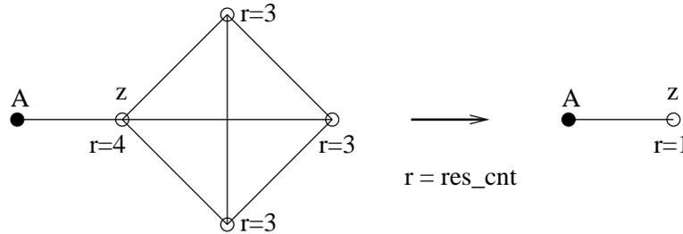
The parameter **delete\_dangling** is added to the code of function *reducArtDegree* to eliminate dangling nodes. Note that a dangling line node is also not eliminated when **min\_art\_degree** is  $\leq 2$ . Thus **delete\_dangling** must overrule the art. parameters.
