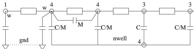
The resistor gets a moment, this is a capacitor element without cap value. The nwell group contains now only one node, with only capacitors connected. It is maybe not a good idea to eliminate this last nwell node. After elimination we get:
