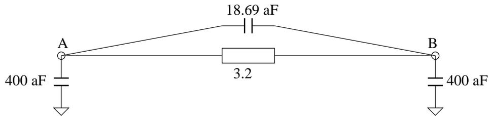
You see that the 600 aF couple capacitances have a small effect (+ 0.69 aF) on the resulting couple capacitance between nodes A and B.
