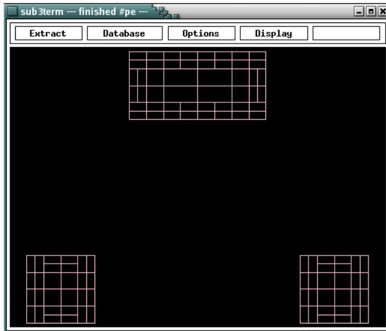
The accuracy of the extraction result is depended of the mesh you chose. And, how finer the mesh, how more computation time is needed to calculate the result.
