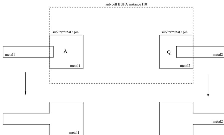
When no sub terminal layout must be added to the top cell layout, the designer has the possibility to use sub terminals which has no dimension. For example, when the sub terminal element has no height and/or width the terminal has no dimension. In that case a connection to the top level layout is only made, when the sub terminal position touches or lays inside the top level mask element.
