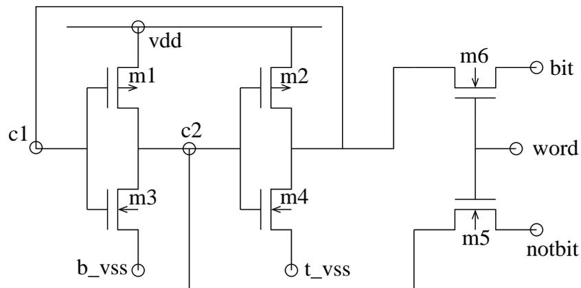
Note that there are couple capacitances between almost all nodes of the circuit. This happens, because the chosen be\_window is  $2\mu m$  width. Each node has also a couple capacitance to the ground plane (node GND).
