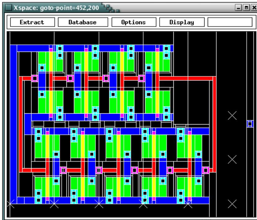
Note that not all strip edges can be shown, because no tile edges are generated. You see on the design top side some tile edges to infinity, which are from the strips.
