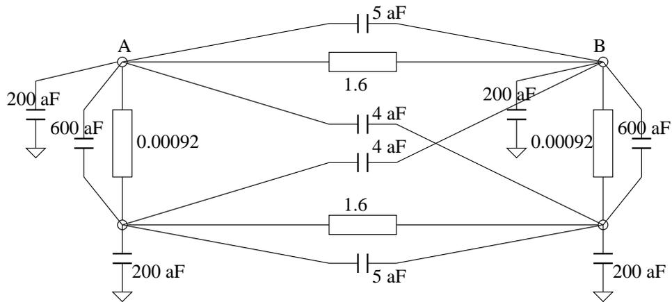
After reduction, the following network is the result of the -rC3 extraction:
