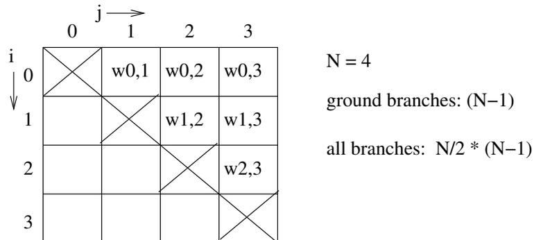
For the ground branches, only the weights for  $i=0$  are calculated (for  $N=4 : 3$ ). When the weights for all branches are calculated, then 6 values for  $N=4$ . For example nodeK is connected with 3 neighbor nodes and has a ground connection (cap-value or moment-value) to the ground node ( $n_0$ ):
