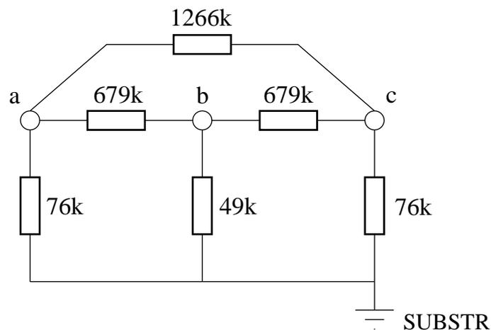
Note that there are substrate resistances between all nodes of the circuit. This happens, because the chosen `be_window` has a width of infinity. Each node has also a substrate resistance to the substrate plane (node SUBSTR).
