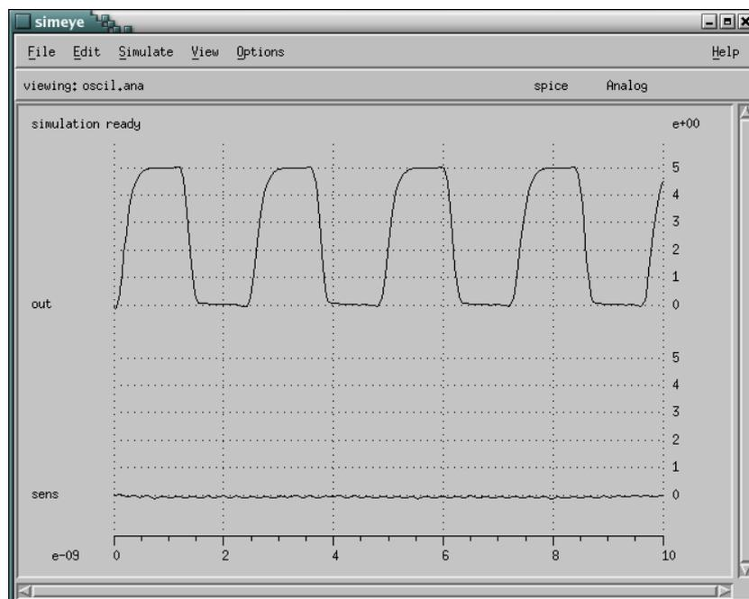
You can zoom-in on the "sens" waveform. Choice the "ZoomIn" item out of the "View" menu. Click with the mouse pointer in the output window, lower left by the "sens" waveform. Draw a rubber box with the mouse around the waveform and click again. To zoom-in even more, set "Detail-ZoomON" item in the "Options" menu. To see the individual waveform points, choice "Values" in the "View" menu.
