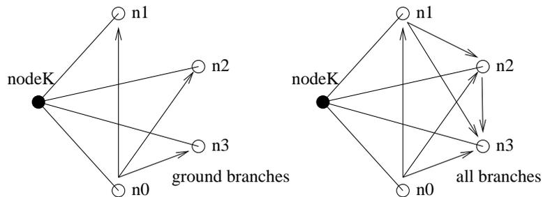
The resulting weight of nodeK is default the square-root of the biggest calculated weight, but below are all possibilities given:
