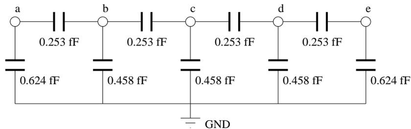
Note that there are no couple capacitances between conductors (a, c), (b, d) and (c, e). This happens, because the chosen `be_window` is  $1\mu m$  width, and the distance between these conductors is more than  $1\mu m$ . Note that the "Space 3D Capacitance User's Manual" shows also the capacitance values in a table for other values of the `be_window`.
