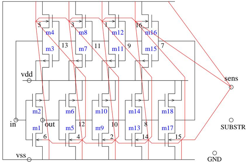
Note that the red lines are substrate resistors. The transistor bulks and substrate contact regions are substrate terminals. There are not substrate resistors between all substrate terminals, because of the interpolation method and the used Delaunay triangulation. However, each substrate terminal has a substrate resistor to the substrate node SUBSTR. When you use the visualization tool Xspace, you can draw an image with the substrate resistors (see below). Type:
