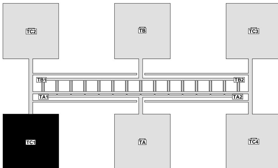
We will study the  $Y_{12}$  between port TA and TB. The ports TC<sub>x</sub>, where x is a number, impose a ground-signal-ground structure. The black pad with port (terminal) TC1 is connected to the substrate, the others are galvanically connected to TC1 but are floating above the substrate. Ports TA1, TA2, TB1, TB2 are connected to TA or TB respectively.
