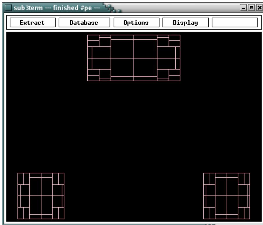
You see three substrate terminals, which are meshed into a number of area's. The complete area of terminal "a" and "c" is  $1.0\mu m^2$ . The area of terminal "b" is  $2.0\mu m^2$ .
