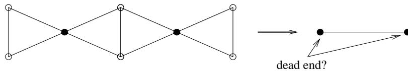
Note that function *calc\_art\_degree* does not compute the **real** articulation degree. It does not take interconnect loops into account and does not find an art. degree of 1 for the following cases:
