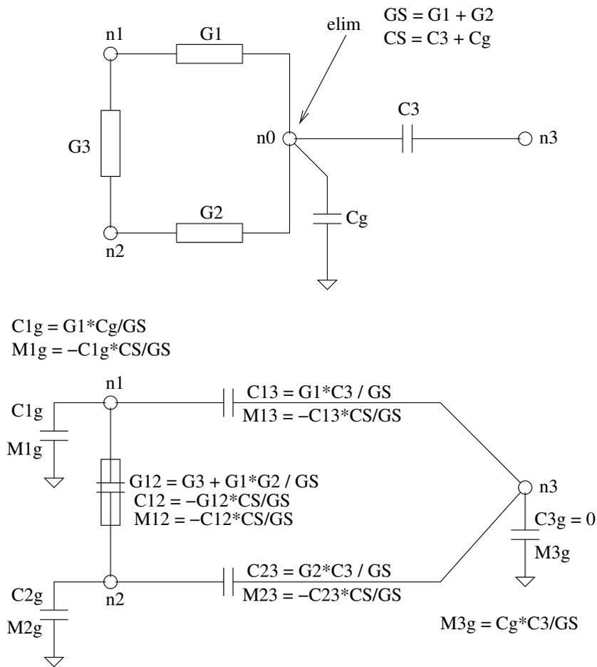
When nodes n0, n1 and n2 are in another group than node n3, you see that the elimination of node n0 has impact on the node n3 of another group. That node gets more coupleCap elements and gets a groundCap. Note that this groundCap has only an extra moments value. Thus a grounded branch for n3 is created via a coupleCap to another group.
