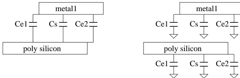
Not all coupling capacitances are folded to the ground node. When the node group of the poly silicon conductor is connected with the node group of the metal1 conductor, then the coupling capacitances are omitted.
