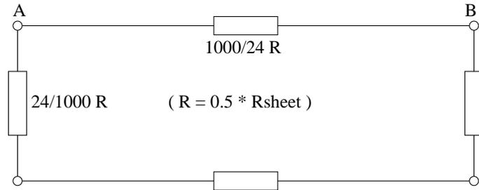
For a Rsheet of 0.077 Ohm/square (using parameter low\_sheet\_res=0.05) the following resistor network is the result:
