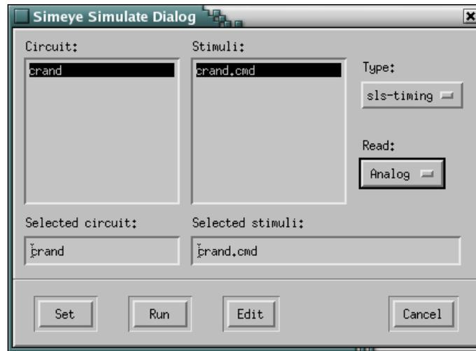
In the dialog window, choice simulation "Type: sls-timing" and for "Read: Analog". Now, start the switch-level timing simulation by clicking on the "Run" button and wait for simulation results. Below, you see the output waveforms.
