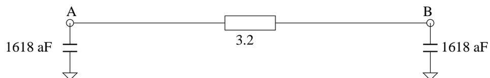
You see that the 600 aF couple capacitances have a big effect on the ground capacitances when we do an extraction with options -rc3.
