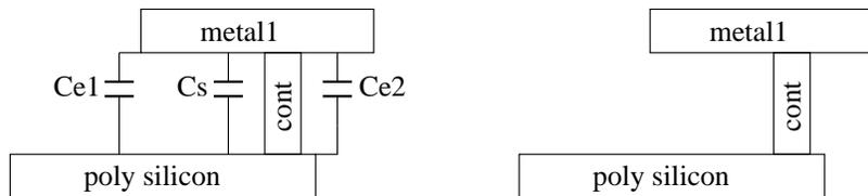
However, capacitances to the SUBSTR node are not omitted, these capacitances are always connected with the GND node:
