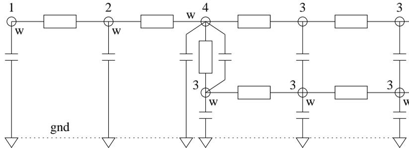
Thus it is possible that nodes with a weight are first eliminated and that makes nodes without a weight possibly more important (giving it a weight). Note that a ground capacitor is also not counted for the degree. Therefore it is maybe better to add an extra priority queue position for a weight  $> 0$  as follows:
