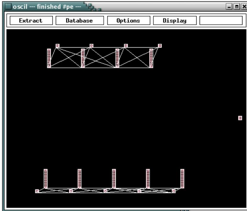
Use hotkey 'i' to zoom-in on the cursor position, to show the mesh in more detail. Use the arrow keys to pan around. Use the 'o' key to zoom-out and 'b' key to set the bounding-box view again. Use hotkey 'q', when you want to quit the visualization tool. The following picture shows a zoom-in example:
