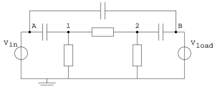
In this circuit,  $C_{A1}$  and  $C_{B2}$  will have values around  $10fF$ ,  $C_{AB}$  will be much smaller, around  $30aF$ . The resistors to ground will have values around  $50\Omega$  and  $R_{12}$  will have a value around  $200\Omega$ .
