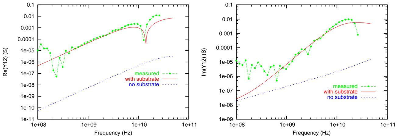
These graphs compare the simulations to the measurements, for the real and imaginary parts of  $Y_{12}$  and for the two networks with and w/o the substrate, respectively. A reasonable match is demonstrated. Please note that the negative peak in the real part of  $Y_{12}$  actually corresponds to a 90-degree phase shift. In the simulation, it can be made almost arbitrarily sharp by increasing the number of simulation points per decade in the file `stim.spc`, line 9.
