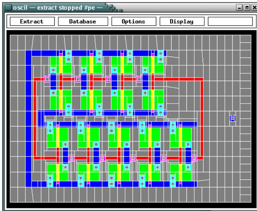
Note that the method is also using the `be_window` size for a substrate bounding box around the design. And that the strips give also extra tile splittings in the y-direction.
