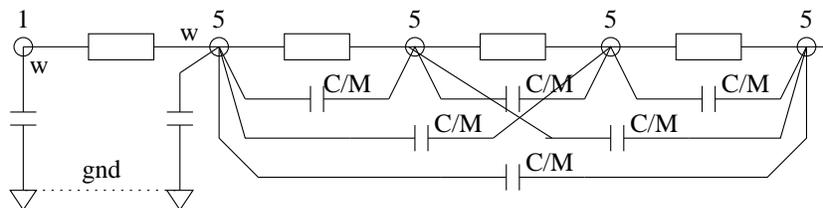
If we don't eliminate the nwell node, there can be many moments parallel to the interconnect resistors. Note that if we make the nwell area low res, then we don't have these moments. However, if we eliminate the nwell node, there can be many capacitors parallel to the interconnect resistors.
